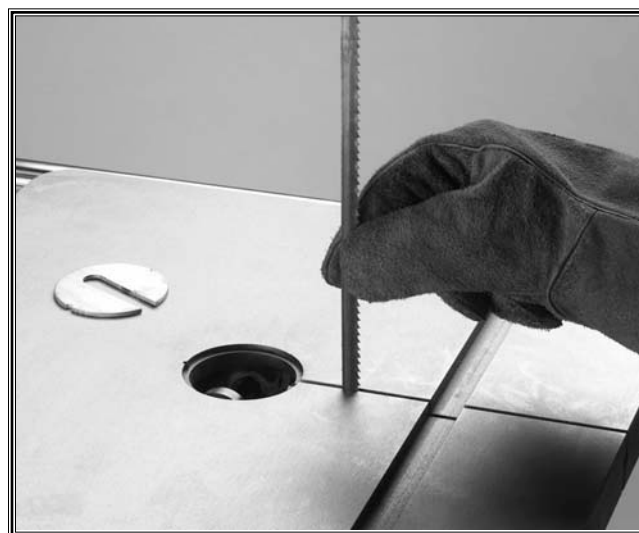
Figure 30. Sliding blade through table slot.
